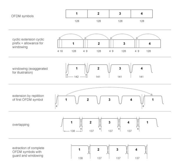
The number of samples used for windowing depends on the cyclic prefix length, normal or extended, and the number of resource blocks. The number of samples is chosen in accordance with the *maximum* values implied by tables F.5.3-1 and F.5.4-1 in [1].
