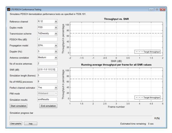
"Analyze Throughput for PDSCH Demodulation Performance Test"
