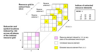
The following diagram shows the extraction process for a 4D channel estimate grid, grid, with NRxAnts = 3 and P= 2. In this case, P is the number for antenna ports. The 4D resource grid consists of P *M*-by-*N*-by-*NRxAnts* arrays, each associated with an antenna port. Resource elements are extracted from all planes within these arrays.
