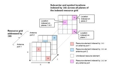
used to extract resource elements address the resource grid with P = 2. In this case, P is the number of antenna ports.
